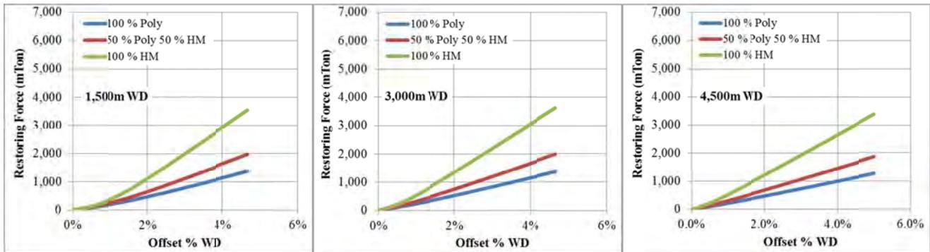
Figure 5. Restoring Force curves as a function of Normalized Offset
