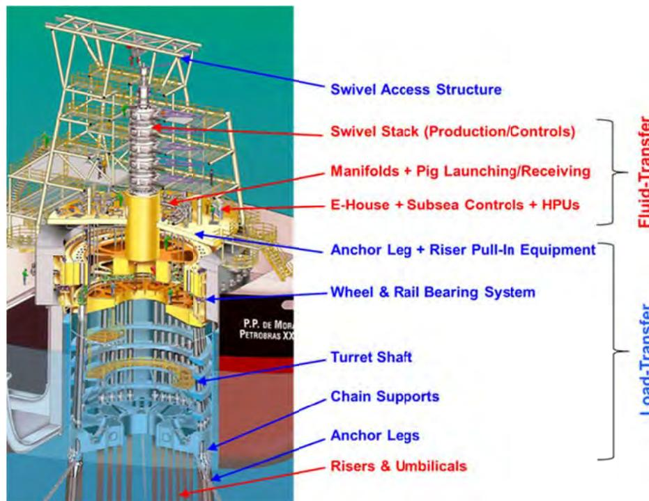
Figure 1. Schematic showing Main Features of an Internal Turret Mooring System
