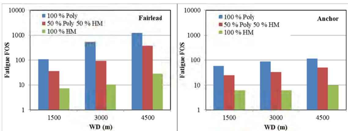
**Figure 7. Results of Fatigue Analysis**
