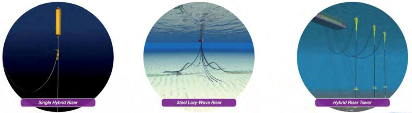
Figure 2. Coupled and Uncoupled Riser Systems (courtesy of Subsea 7)
