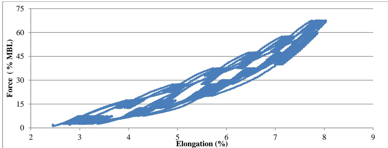
Figure 3. Stiffness test of polyester rope
