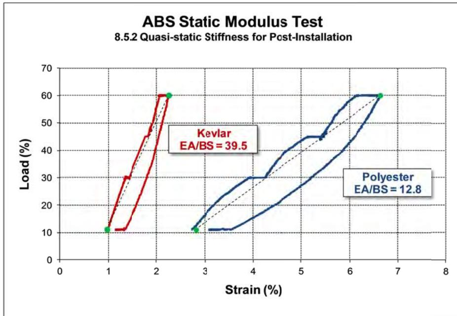
Figure 4. Comparison between Quasi-Static Stiffness of a Kevlar and Polyester Rope (courtesy of Whitehill Manufacturing).
