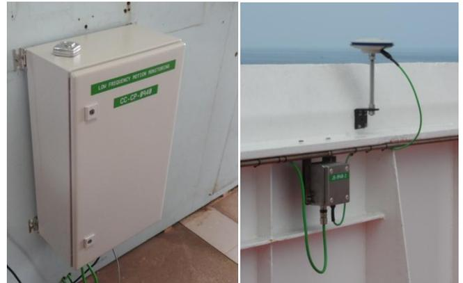
Figure 2. A Position Monitoring System (PMS) installed on the on wheelhouse of an FPSO
