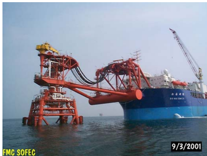
Fig. 1 Tower-yoke mooring system for CNOOC QHD 32-6 FPSO
