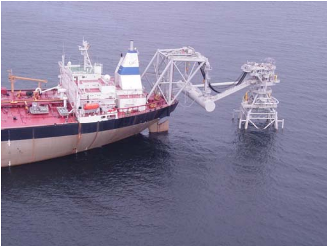
Fig. 2 Tower-yoke mooring system for ESSO Chad FPSO
