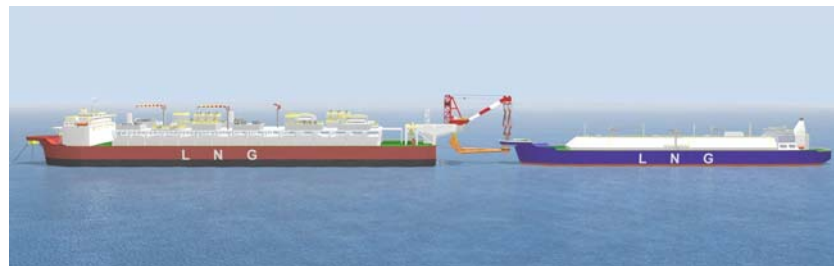
Figure 4 Revolving Boom Tandem Loading System
