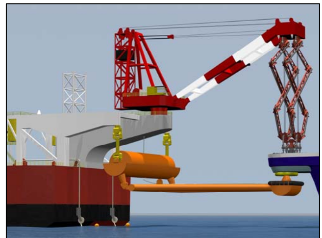
Figure 5 Revolving Boom Tandem Offloading System
