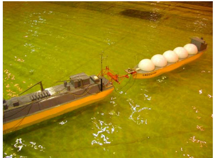
Figure 8 LNG carrier berthing operation tests
