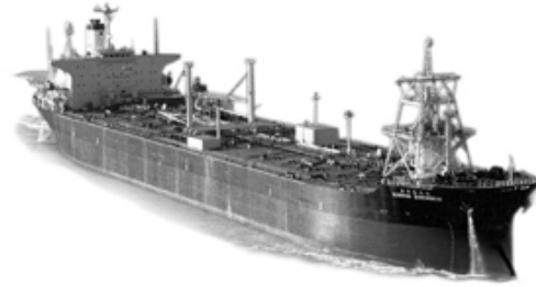
Image 2 Disconnectable turret for JHN, People's Republic of China - Lufeng 13-1 Field, for Nan Hai Sheng Kai FSO
