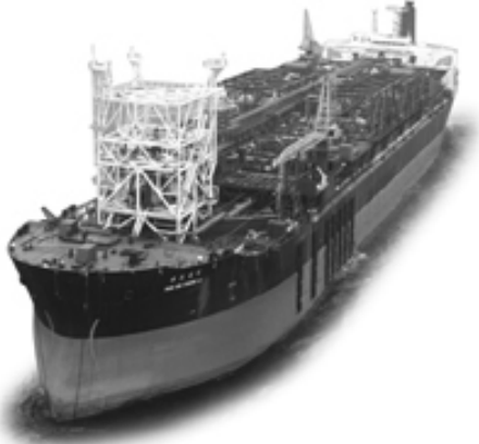
Image 1 Fixed turret for Amoco Orient Petroleum Co., People's Republic of China, Liuhua 11-1 Field, Nan Hai Sheng Li FPSO
