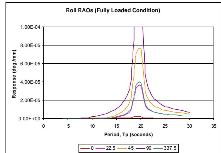
Figure 12 FPSO Roll response in head sea (Fully loaded condition)
