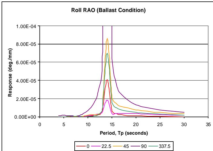
Figure 11 FPSO Roll response in head sea (ballast condition)
