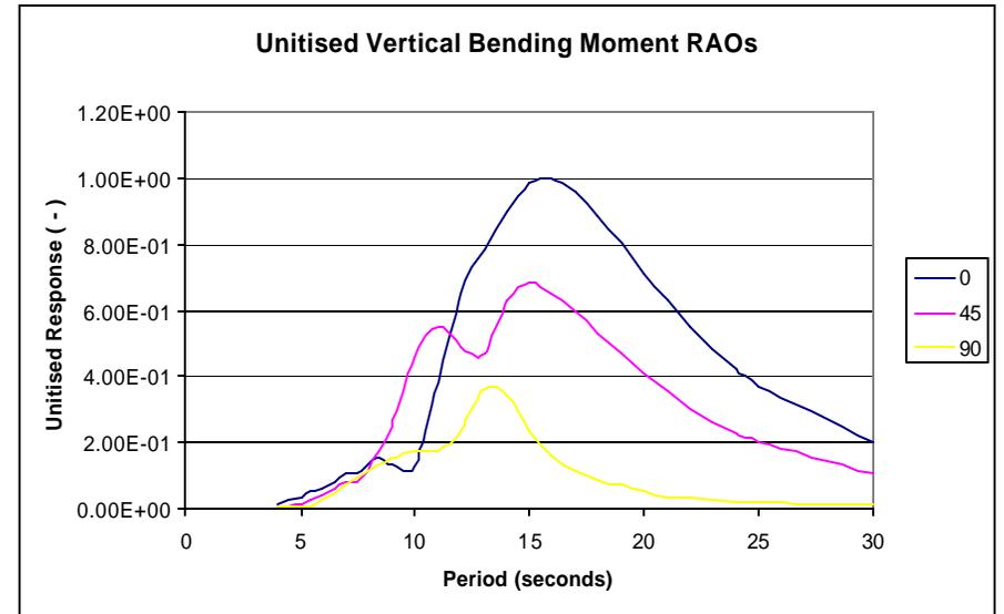
Figure 10 Unitised FPSO Vertical Bending Moment RAOs
