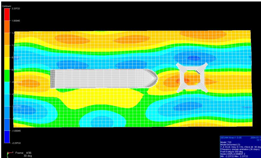
Figure 17 Visualization of Hydrodynamic Interaction
