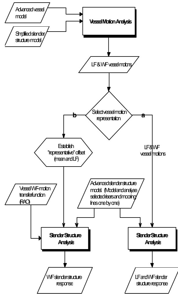
Figure 18 Typical Flowchart for Coupled Analyses
