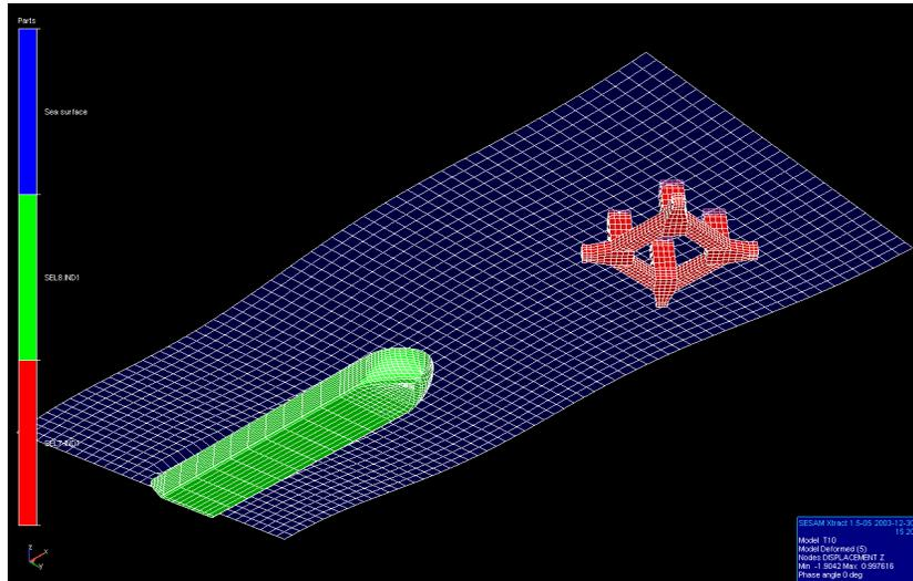
Figure 13 FPSO and DTU (TLP) seen from below
