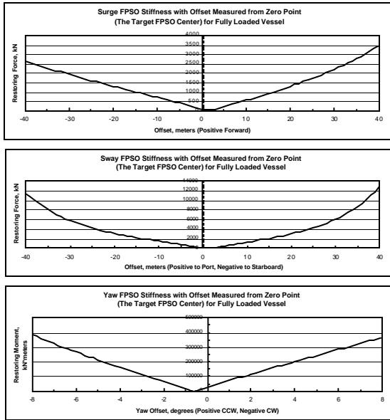
Figure 5 Mooring System Stiffness Curves for Spread-Moored FPSO
