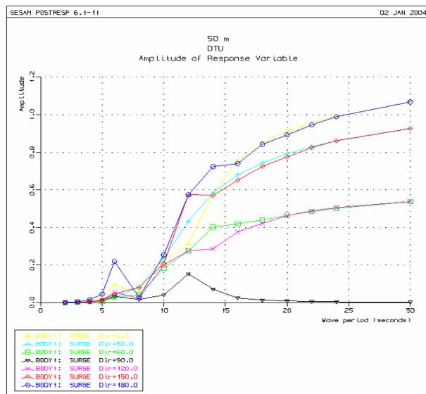
Figure 15 DTU Surge, 50 m Separation
