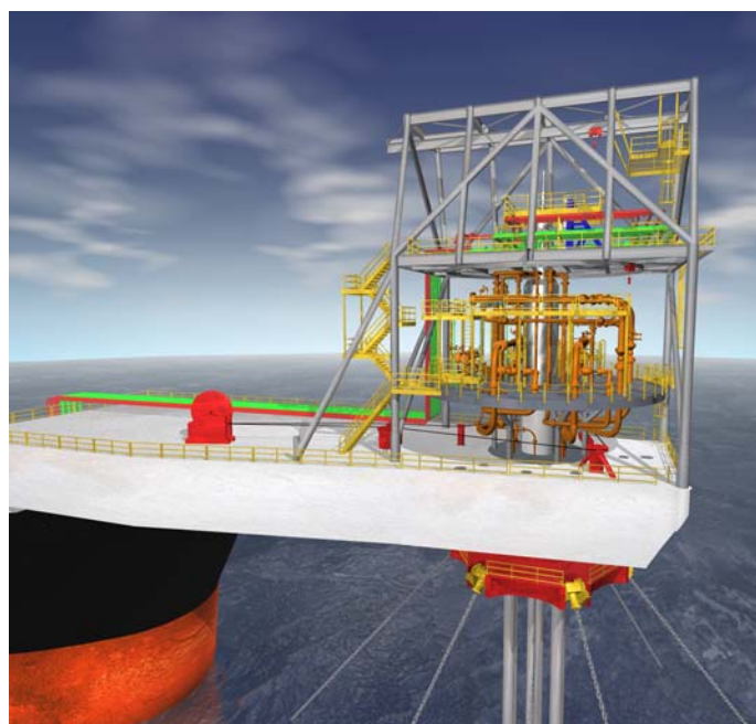
Figure 2: External Turret Mooring System
