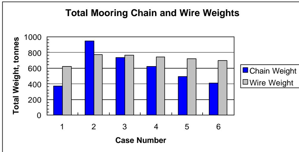
Figure 2. Bar chart showing the total chain and wire weights required for Cases 1 through 6 in order to meet the current API RP 2SK guidelines.
