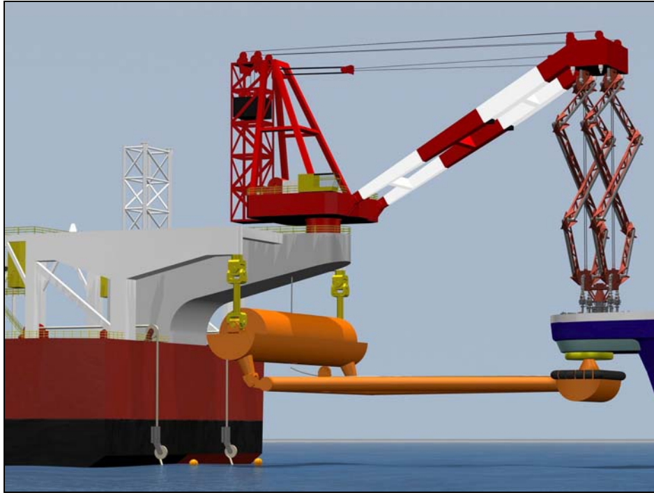
Figure 12: Revolving Boom Tandem Offloading System
