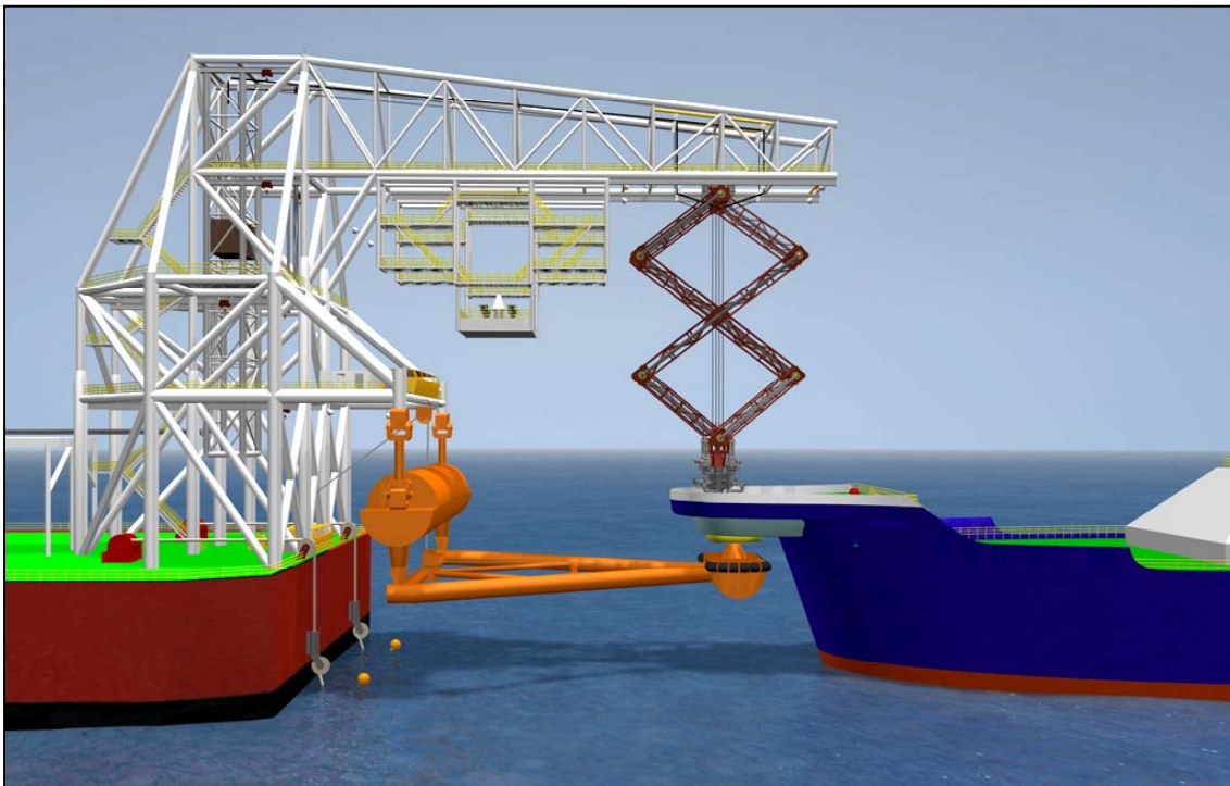
Figure 9: Stationary Boom Tandem Offloading System in Operation
