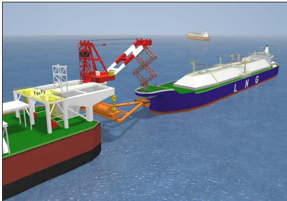
Figure 11: Revolving Boom Tandem Loading System
