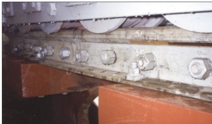
AmClyde-type wheel and rail bearings (above) can be assembled into large-diameter bearings (top right).
