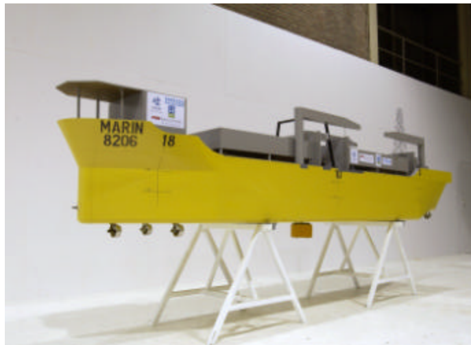
Figure 5. DP FPSO model with disconnectable buoy
