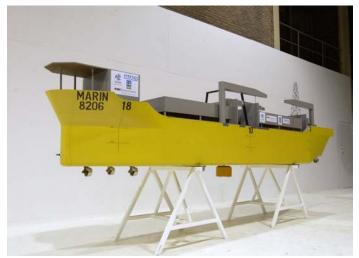
Figure 5. DP FPSO model with disconnectable buoy
