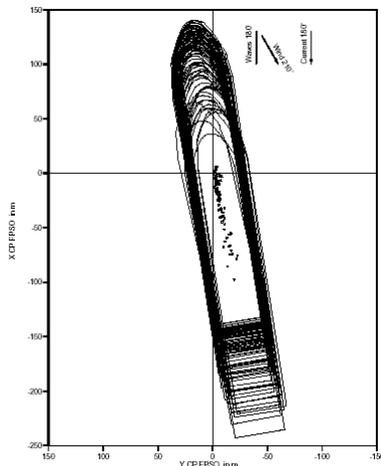
Figure 12. DP positioning in 10-Year hurricane conditions
