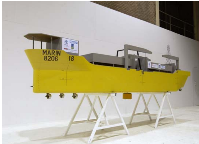
Figure 5. DP FPSO model with disconnectable buoy
