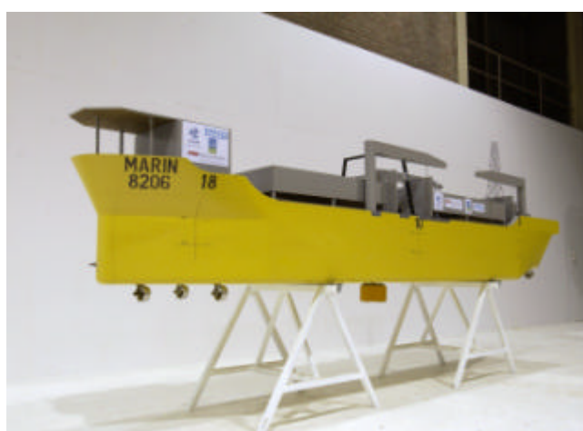
Figure 6. DP-FPSO model with disconnectable buoy
