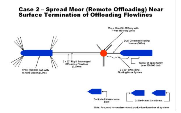
The FPSO spread mooring system would be fifteen (15) lines with the top chain section of 150 meters of 119mm R4 studless, center wire section of 2,000 meters of 119mm SPR2 unsheathed, and the bottom chain section of 150 meters of
