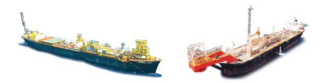
Please note that external turrets are not recommended for this example of the average West Africa deepwater field because current external turret designs are limited to approximately a capacity to twenty (20) risers. This limitation is necessary or otherwise the loads on an extension on the bow or stern to attach the external turret become too large to be economically and technically viable.
