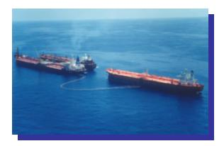
Specifically for West Africa, side-by-side offloading is not an acceptable method due to long swells from the south and uncorrelated wind and current events. The region is also subject to wind squalls with velocities up to 30 m/s that can develop very quickly, which is a high risk for this method during the offloading operation. There is also a high risk of collision during offloading due to the close proximity of the FPSO and tanker of opportunity.
