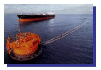
Due to the tanker of opportunity weathervaning about the remote CALM terminal, it needs to be located in an area where the tanker of opportunity is free to move through a 360-degree arc without any risk of collision with the FPSO or any other field traffic. The present standard clearance in the West African region for the terminal is one nautical mile (approximately 1,850 meters).
