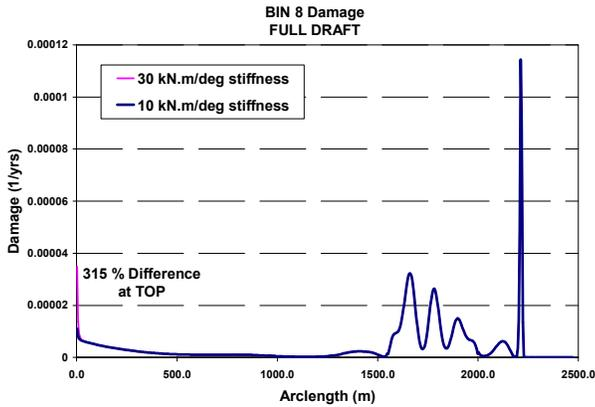
Figure 13. Fatigue Sensitivity to Flexjoint Stiffness
