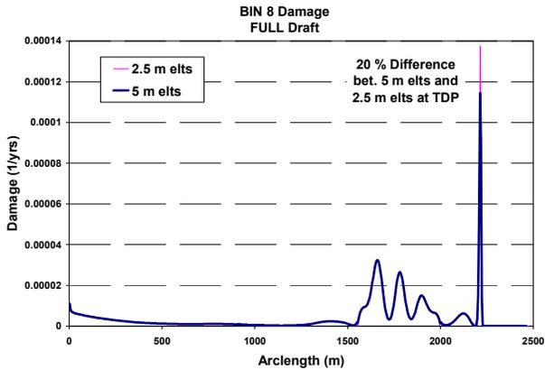
Figure 12. Fatigue Sensitivity to Element Size
