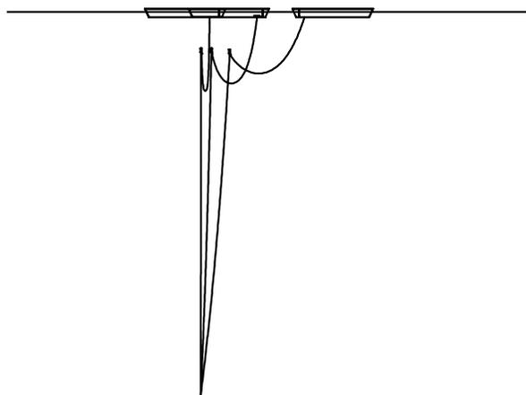
Figure 9. SLHR in near, mean and far positions
