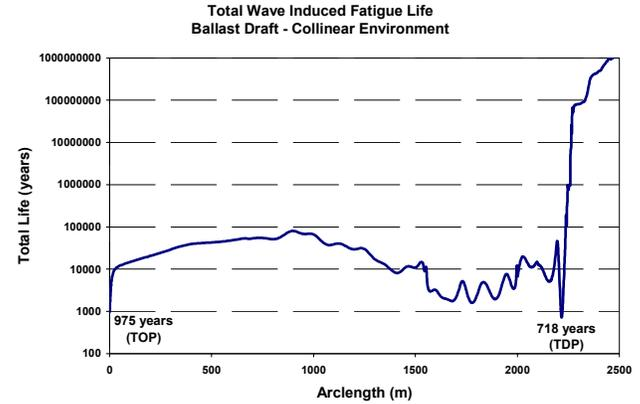
Figure 11. Wave Induced Fatigue Life Along SLWR
