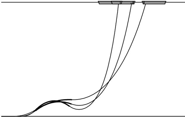
Figure 1. SLWR in near, mean and far positions
