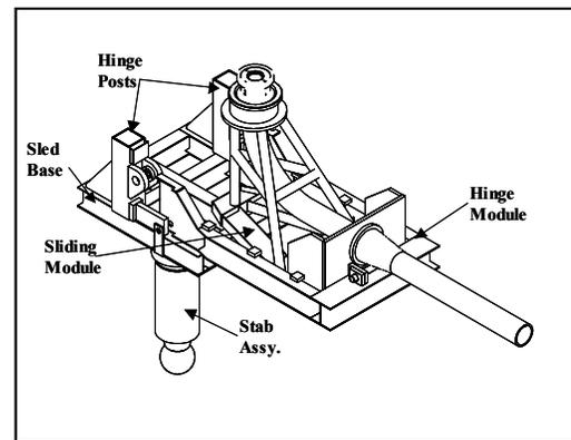
Figure 5. Stab and Hinge Over Assembly
