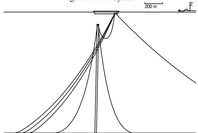
Figure 3. TLR System Layout
