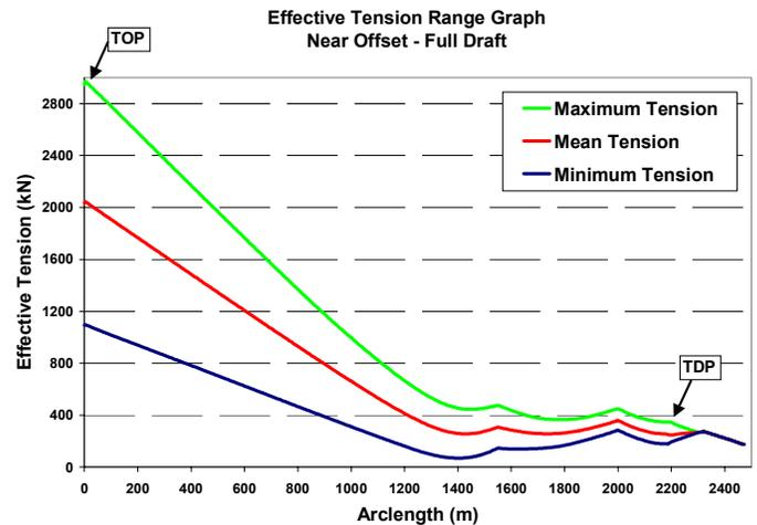
Figure 10. SLWR Effective Tension Range Graph
