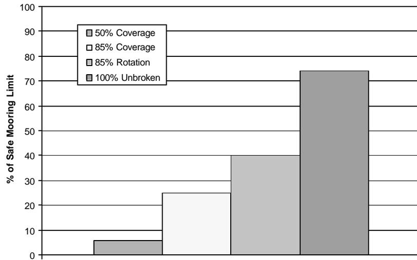
Figure 8 – Pack Ice Loads on FPSO as a function of Surface Coverage
