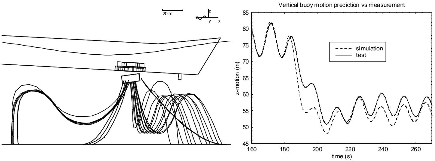
Figure 9 – Comparison of Computed and Measured Free Fall of Spider Buoy in Maximum Disconnect Environment
