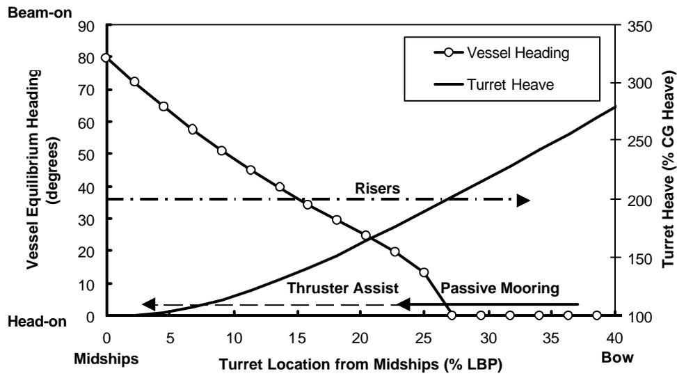
Figure 3 – Impact of Turret Location on Vessel Equilibrium Heading
