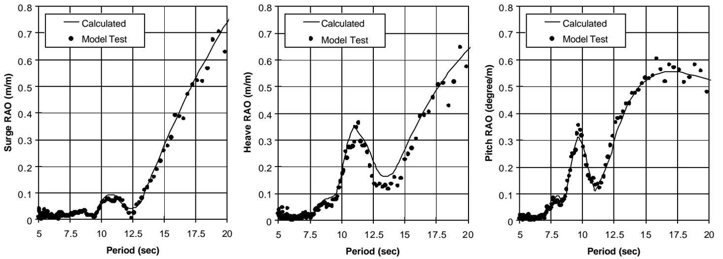
Figure 6 – Comparison of Computed and Measured Vessel RAOs for Head Seas
