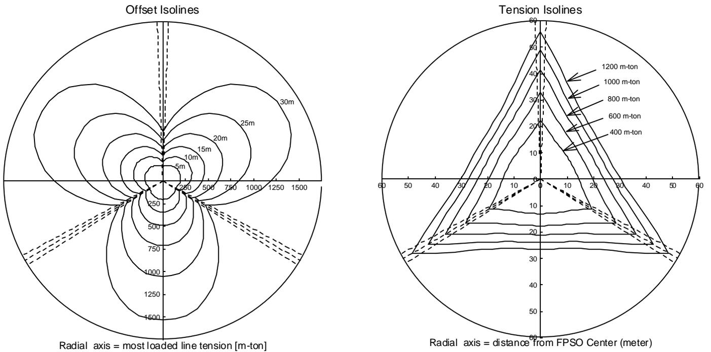
Figure 4 – Offset and Most Loaded Line Tension Isolines as a function of Mooring Orientation
