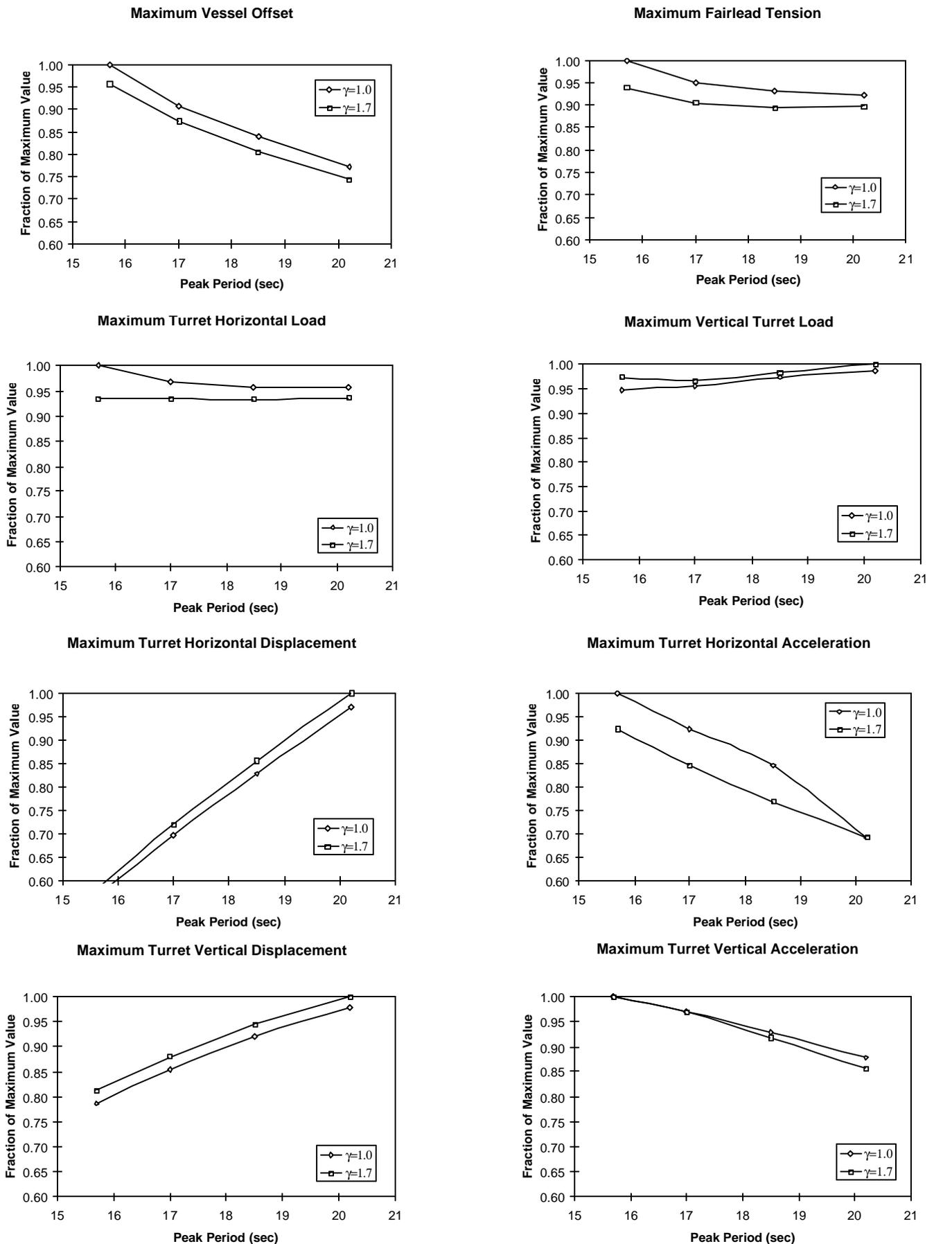
Figure 5 – Sensitivity of FPSO Response as a function of Wave Spectral Period and Peakedness Parameter
