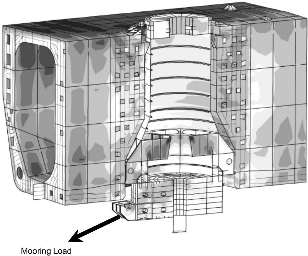
Figure 7 – Stresses and Deflections from Finite Element Model of Turret and FPSO Vessel in 100-year Storm Environment
