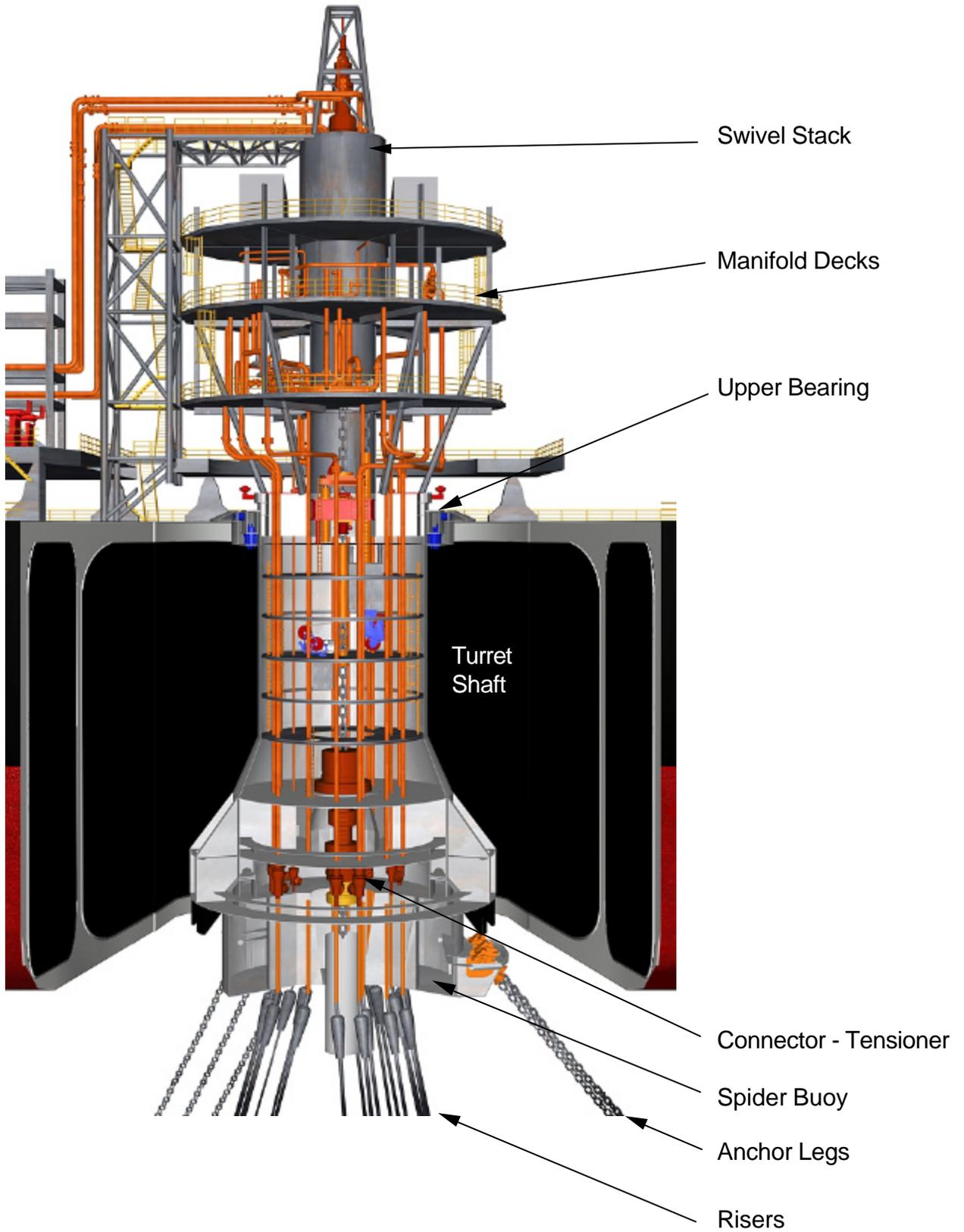
Figure 2 – Schematic of Turret Mooring System
