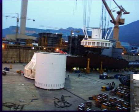
Lower turret module (TS1) inserted in ships moon pool keel block
