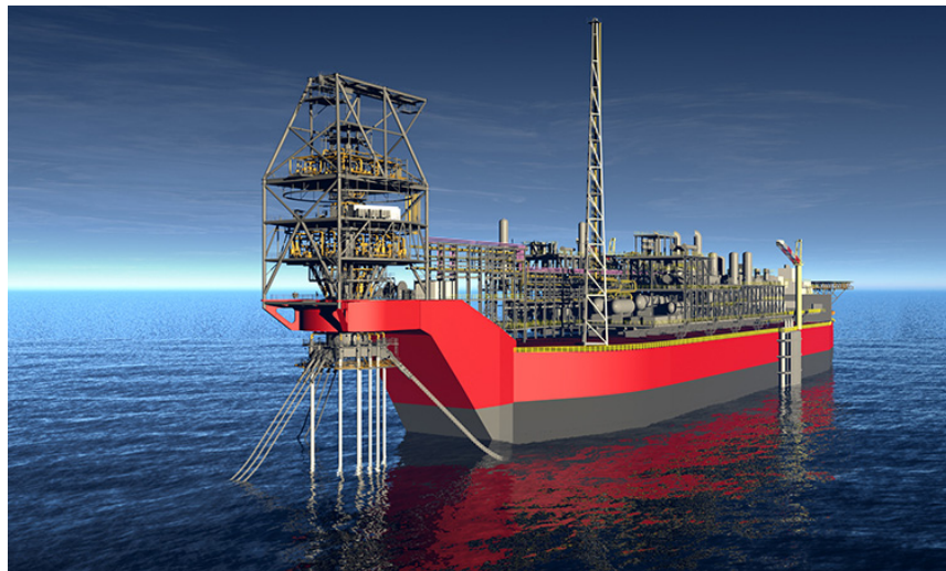
Rendering of the Sangomar Field Development FPSO with SOFEC's External Turret Mooring System (Image courtesy of SOFEC)
