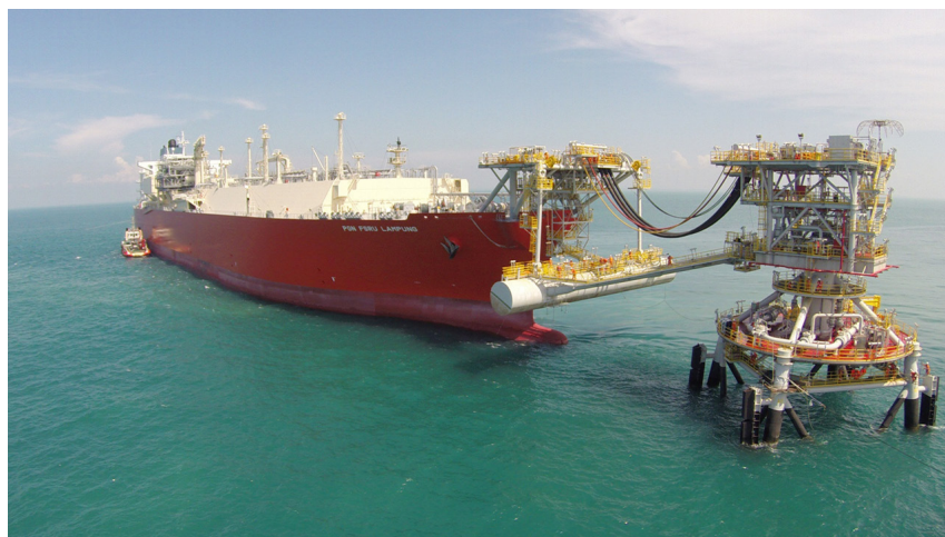
Figure 2. The Tower Yoke moored Hoegh Lampung FSRU (image courtesy of Hoegh LNG).
