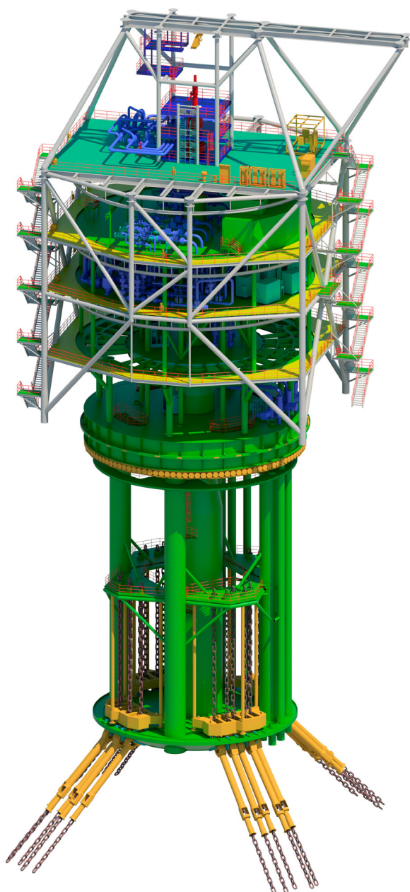
Figure 5. The SOFEC Very Large Turret (VLT).
